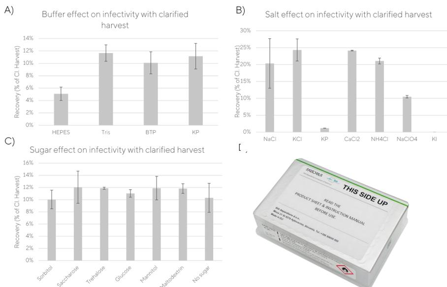
Figure 1: Results from buffer optimisation of process for lentiviral purification. Effects of different A) buffers, B) salts, and C) sugars were tested for buffer optimisation. D) Photo of CIM QA 0.05 mL Monolithic 96-well Plates (6 µm channels), which were used for the buffer optimization and DoE.
